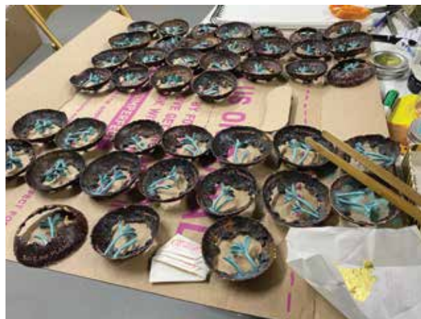
Fig 2d. Apply green patina with a burner, engrave the letters, splay an anti-tarnish coating, and finally apply gold leaf
