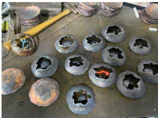
Fig 2b. Use a Tig welder to make holes while melting the center. Melt randomly from the edges as well
