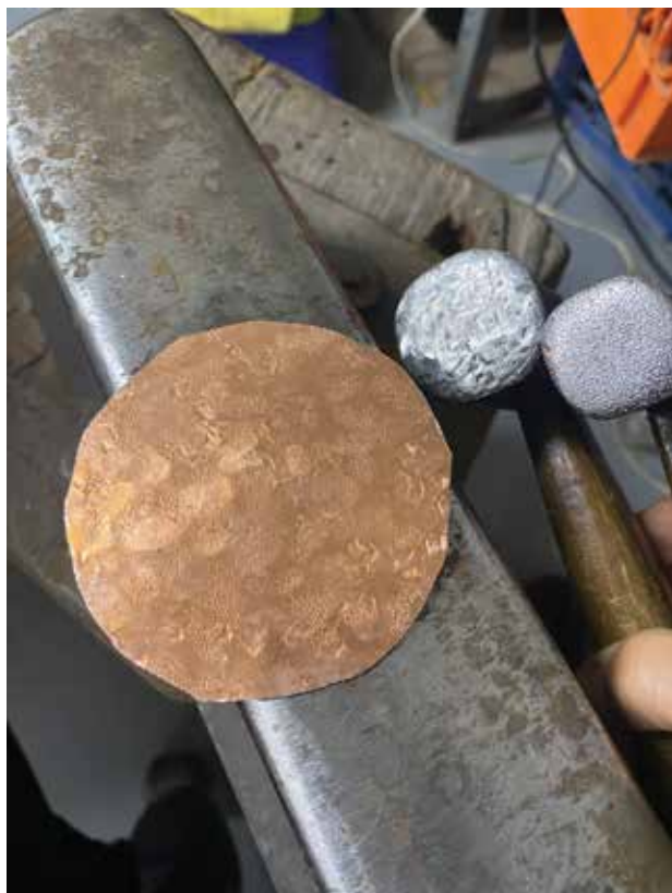
Fig 2a. Cut out the copper plate and apply a pattern to the copper plate with a pattern hammer
