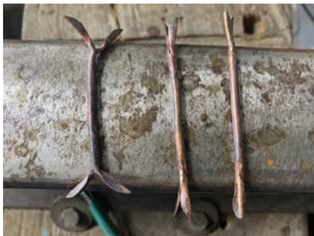
Fig 2c. Sprouts have formed the shape with a chisel and hammer on the anvil to make one sprout on each end
